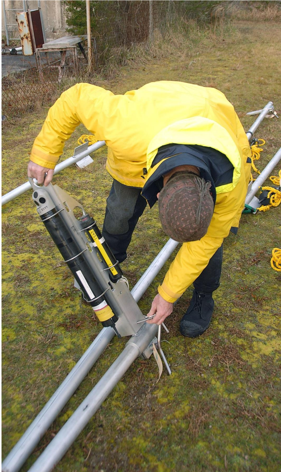
Figure 3. A U.S. Geological Survey employee mounting a cantilever arm holding an Aquadopp (current profiler using Doppler technology) and pinger onto a jet pipe. Photograph by Don Bowers.
